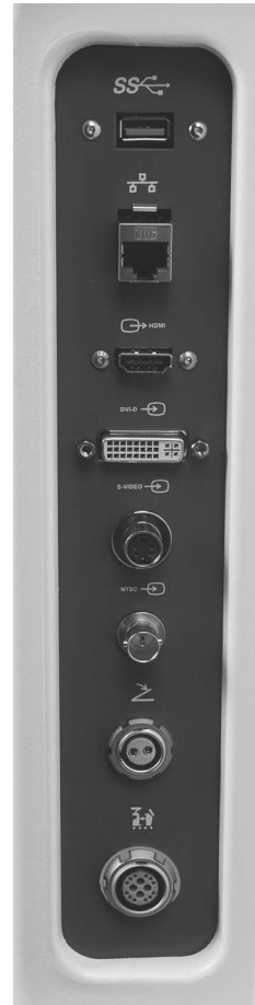
Figure 15: Main cart communication I/O panel
